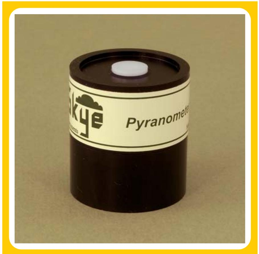
The SKS 1110 Pyranometer sensor is probably the widest selling unit in the Skye Instruments' range of sensors, with units sold all around the globe. It offers a compact sensor for solar energy measurements and compares favourably with thermopile sensors, offering considerable financial savings.
