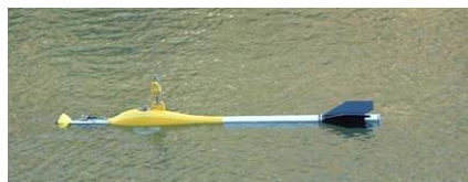
Measurement with current meter type SEBA F1
