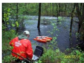
Measurement with Workhorse Rio Grande and Riverboat
