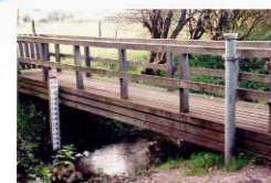
water level measurement with pressure sensor
