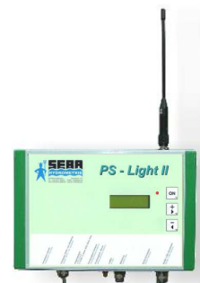
PS-Light-2 with GSM modem and antenna
